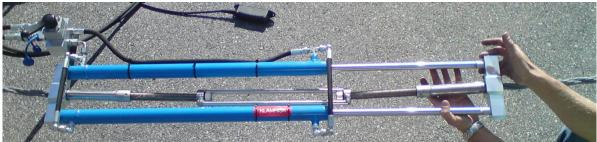
Picture 5. Hydraulic traction device mounted to tensioning unit. Fasten nuts to lock the unit in position.
